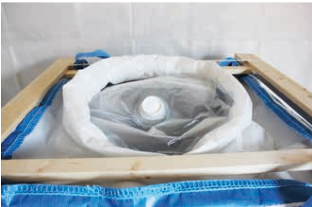
Closed inliner after filling. Afterwards the fabric filling spout will be closed.
