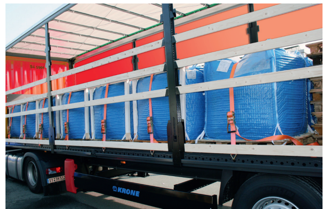
22 INDUTAINER IBCs of 1100 kg each = 24,2 t
